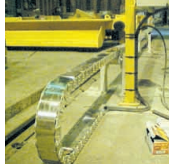
Provides a safe process: Boa steel chain with covers in a steel mill.
