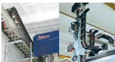
A portal robot equipped with a Cobra chain permits reliable, efficient picking, placing and positioning.
