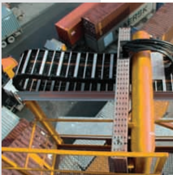
Conductix-Wampfler Cobra energy guiding chain on a port crane.
