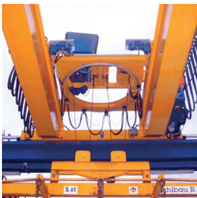
Supply of the turning-crab on an EOT-crane
