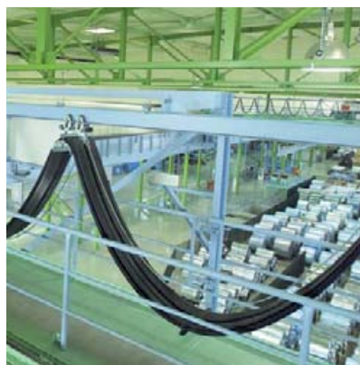
Energy and data transmission on a steel-mill-crane
