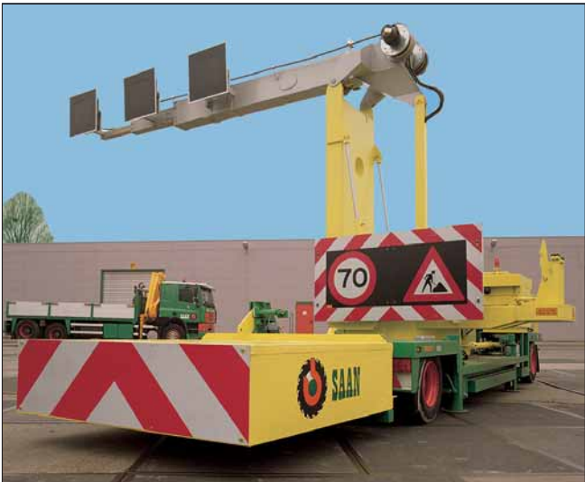
Two spring cable reels in operation on a mobile traffic sign bridge.
