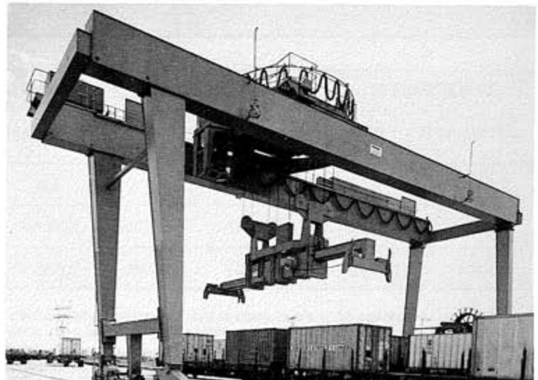
Feed circular current to an underhung revolving jib of a container-portal crane.
