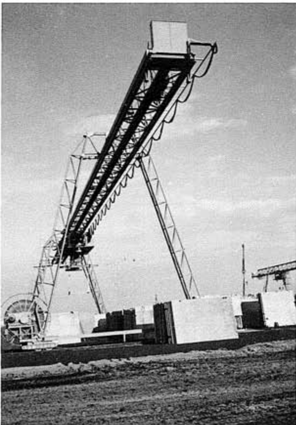
Crab flexible cable system for a stockyard crane.
