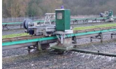
We grow your business! A Walker motorized reel on an outside irrigation system.
