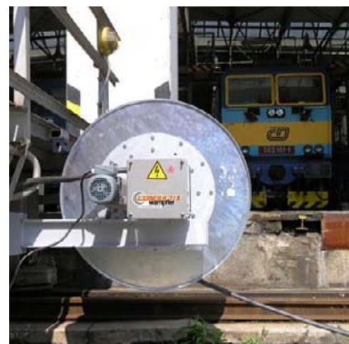
On the track! The Walker motorized cable reel provides main power supply for a railway transfer car.
