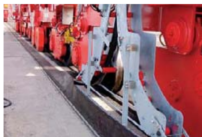
Cable guide on RMG Yard Crane
