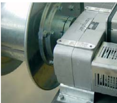
Conductix-Wampfler spur gear with standard motor and magnetic clutch for low to medium torque
