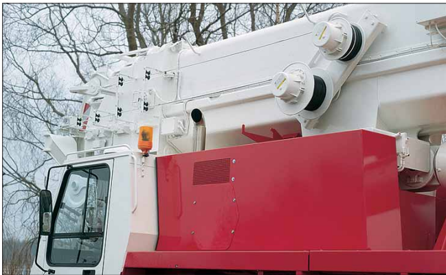
Spring cable reel on a mobile crane for the control of load-level and positioning of the telescopic boom.
