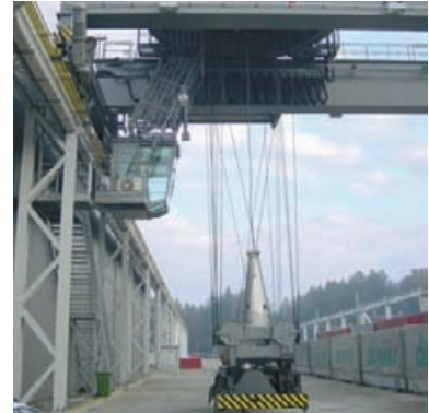
Spring cable reel Stock&Go on a spreader
