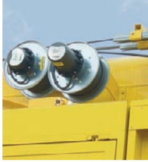
Spring cable reels Stock&Go on a rail mounted mobile crane
